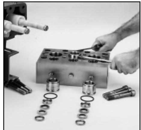
6811, 6821, 6841 Inlet Manifold and V-Packing Cylinder
