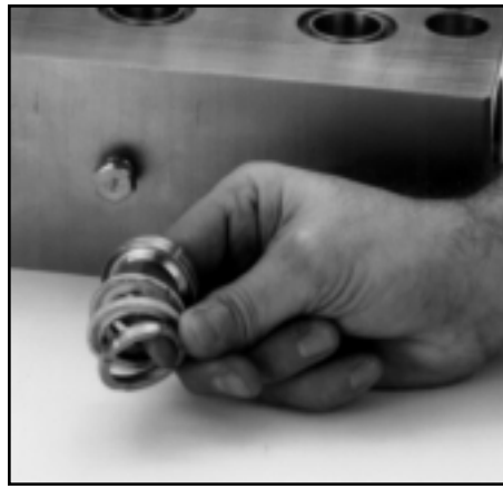
6811, 6821, 6831, 6841 Inlet Manifold and order of Packings
