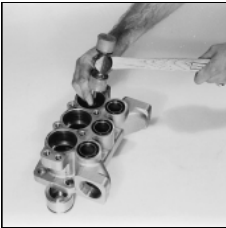
Removing the Inlet Adapter from the Inlet Manifold
